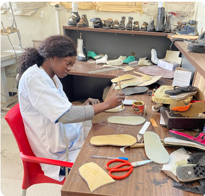
To enhance local mobility solutions, a technician in Senegal creates custom orthopaedic shoe insoles, which are carefully fabricated by hand at the National Orthopaedic Equipment Centre. © CNAO
