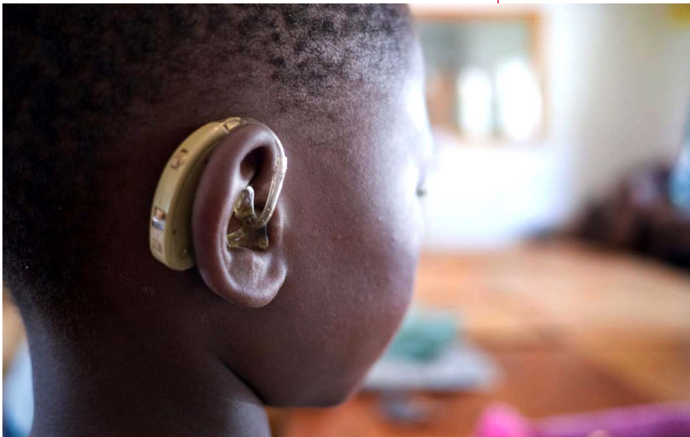
A boy with hearing impairment wears a Solar Ear hearing aid in the eastern city of Mutare, Zimbabwe. The Solar Ear battery charger lasts for 2–3 years and can be used with 80 per cent of hearing aids on the market today. It can be charged via sunlight, household light or a cellphone plug. © UNICEF/UNI174951/O'Donoghue
